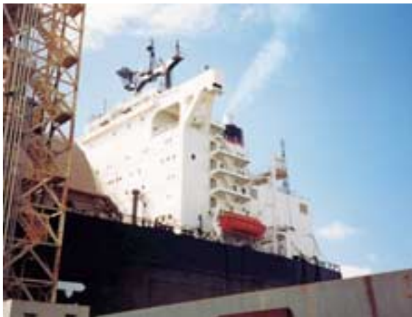
An aesthetic topcoat usually is applied to the topside and superstructure for good appearance.
