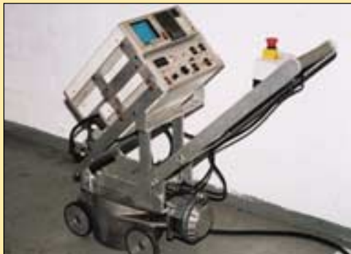
Fig. 2 - Currently available MFL/EC unit
