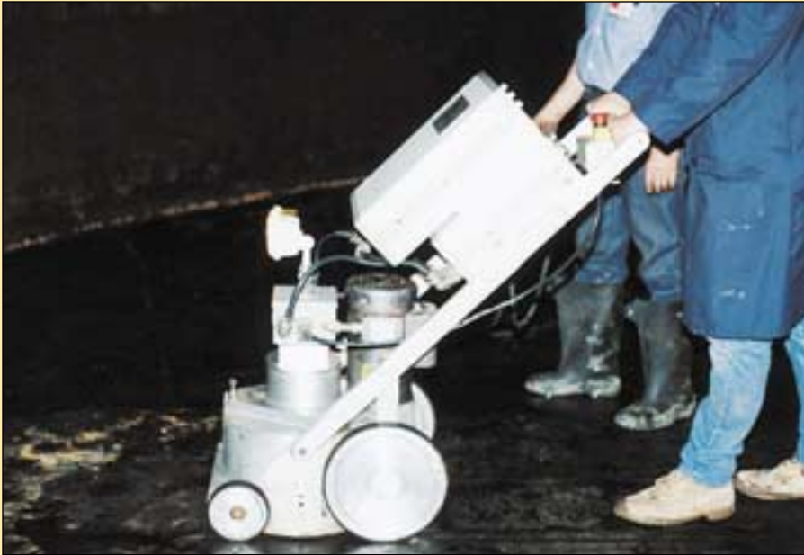
Fig. 2 - Currently available MFL/EC unit
