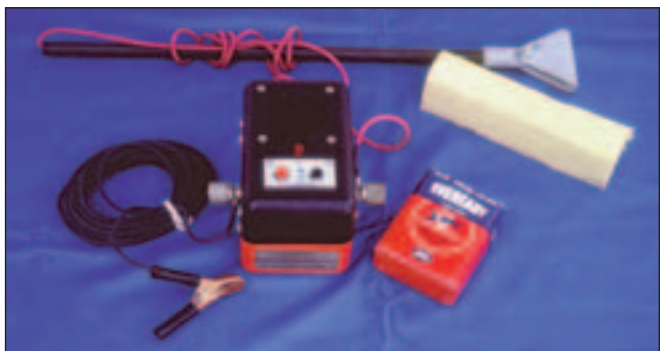
Fig. 1: Low-voltage holiday detector (Photos courtesy of the author)
