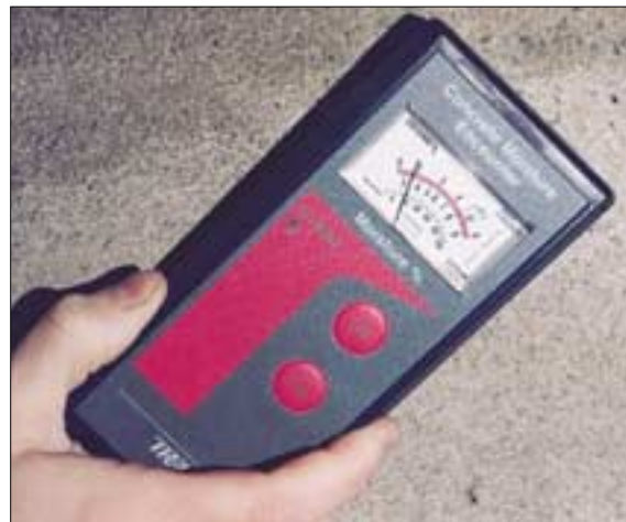
Fig. 2 - Moisture meter for the gel bridge test Photo courtesy of Delmhorst Instrument Co.
