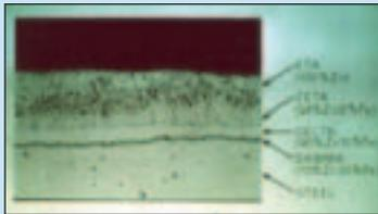
Chemical reactions between the iron in the steel and the molten zinc take place, forming four distinct layers, as shown at left. The gamma layer closest to the steel is 75% zinc and
