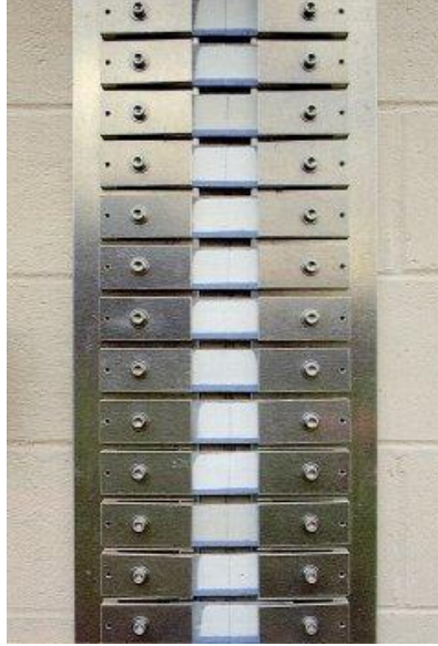
Figure 8. Photograph of the moving wall testing device. Clamps on either side of a vertical expansion joint in a cinderblock wall each hold half of a fiber cement board, connected only by the coating film bridging the gap.
