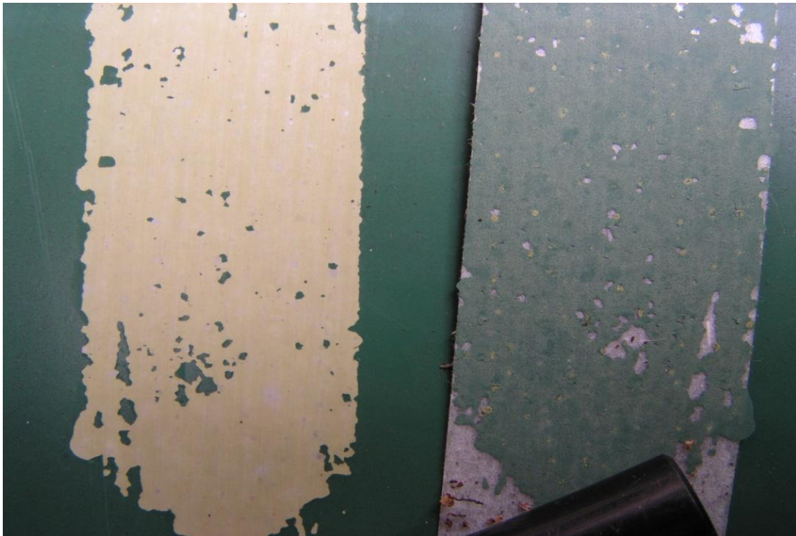
Figure 1: Adhesive tape was applied and removed without any knife cutting. The underside of the tape is on the right, and the area of detached coating is on the left.
