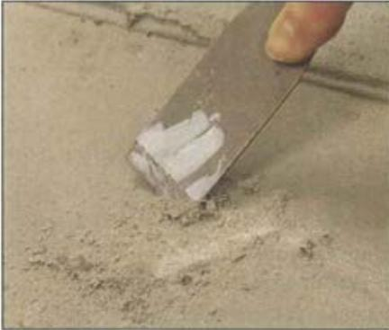
**Fig. 5: Scratching a concrete surface with a stiff blade can also show whether laitance is present. If the blade gouges the surface, laitance is likely present.**
