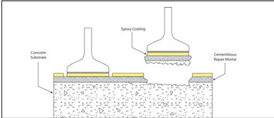
Fig. 2: Tensile strength testing, ASTM D 7234
