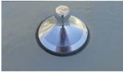
Fig. 4a: Testing surface tensile strength properties using 50-mm-diameter dollies in accordance with ASTM D 7234
