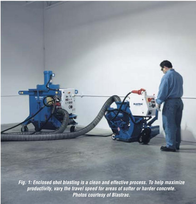
*Fig. 1: Enclosed shot blasting is a clean and effective process. To help maximize productivity, vary the travel speed for areas of softer or harder concrete. Photos courtesy of Blastrac.*
