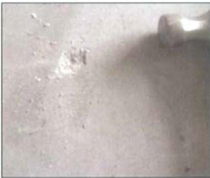
**Fig. 4:** Concrete can be tested for the presence of laitance by lightly striking the substrate with a hammer. Powdered dust in the indentation indicates unsound concrete.
