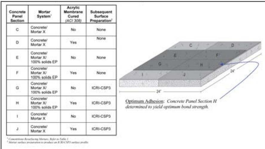
Fig. 5: Bond strength matrix—trowel finished/mechanically profiled
