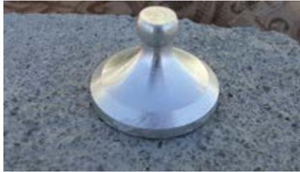
Fig. 4b: Testing surface tensile strength properties of Concrete Control Panel A (SSPC-SP 13/NACE No. 6, ICRI-CSP5 prepared concrete panel) using 50-mm-diameter dollies in accordance with ASTM D 7234.
