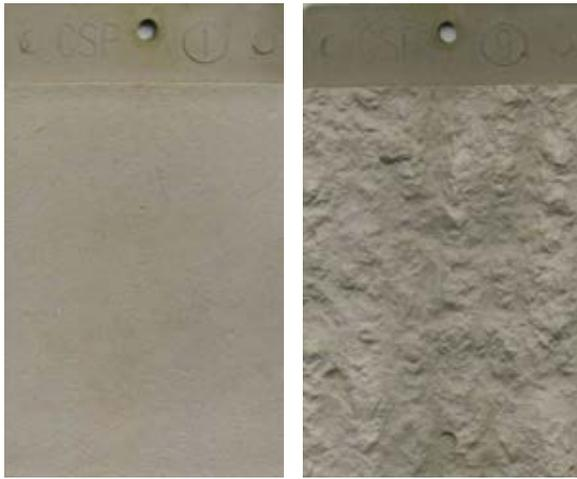
Fig. 1: (left) ICRI CSP 1 (nearly flat); (right) ICRI CSP 9 (very rough)
